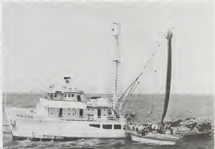
North American purse seiner, with wheelhouse forward and power block for working the net.
